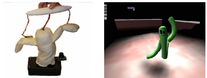
Fig. 2. TUI3D; tangible puppet interface (left) controls the virtual character in the Unreal engine (right).
