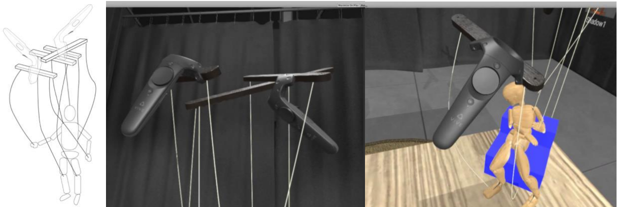
Fig. 6. principle marionette control scheme (left) implemented visible controllers and detaching functionality (middle) controlling the Educational Puppet with different hand controllers (right).
