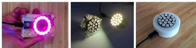
Figure 2. Electronics revision from breadboard model to custom circuit board with digital fabricated platforms.
