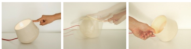
Figure 5. Left, Middle: nudging the lamp to increase light intensity. Right: resting the lamp to dim it.
