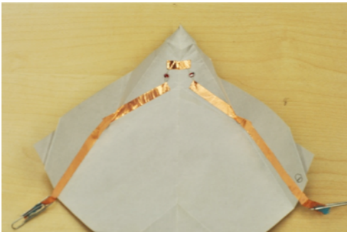
Figure 4: Internals of the origami puppet
