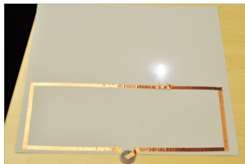
Figure 1: Series circuit with conductive tape
